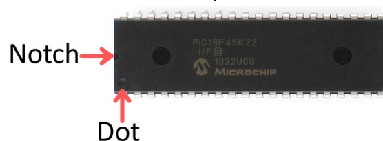
Polarity Marking and Pin Numbering
