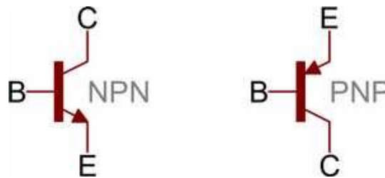
The circuit symbols for the NPN and the PNP Transistors
