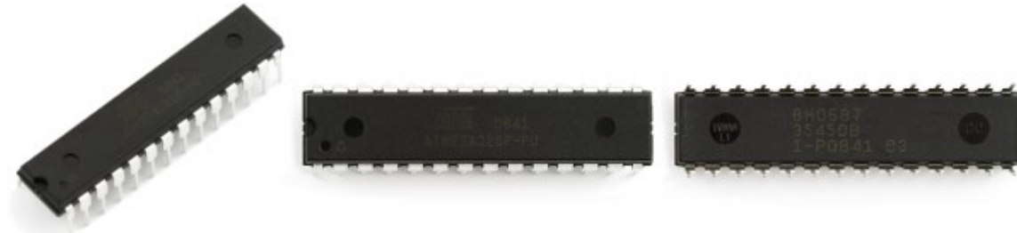
The 28-pin ATmega328 is one of the more popular DIP-packaged microcontrollers.
